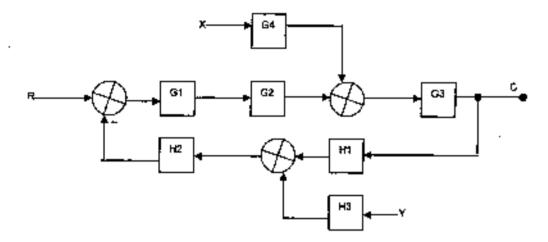
(b) Reduce the given block diagram to its canonical form and hence obtain the equivalent [6] transfer-function.
