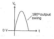
This is an example of the output swing for a \_\_\_\_\_ push pull
